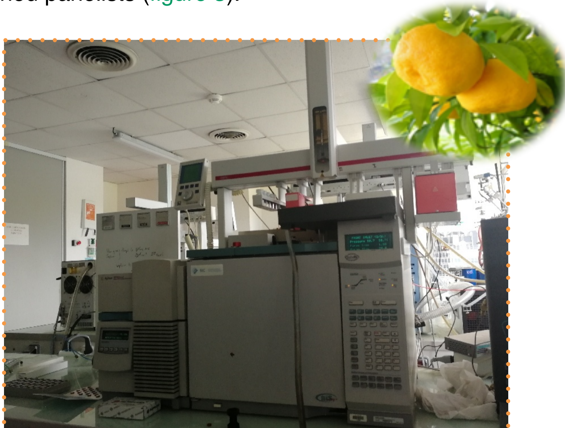
Figure 2. (SPME) combined with gas chromatography/mass spectrometry (GC/MS).
