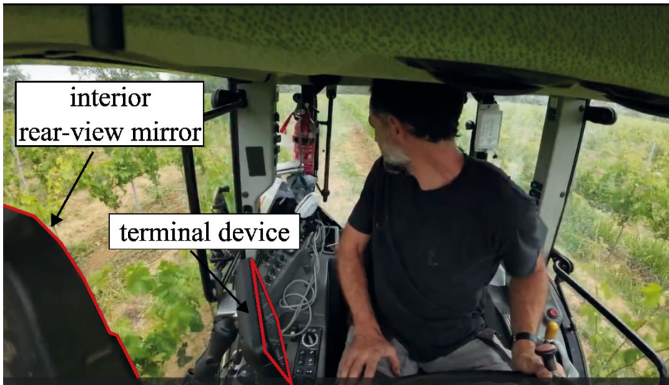
Figure 3. Example of an image grabbed from the camera located inside the tractor cab during the weeding operation. It shows the case of the driver's backward gaze to verify that the rear-mounted tool is correctly aligned between the vine rows, preventing potential damage to the plants, and that the weeding quality is good enough.
